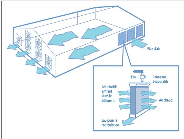
Illustration 14. Pad cooling en ventilation tunnel
