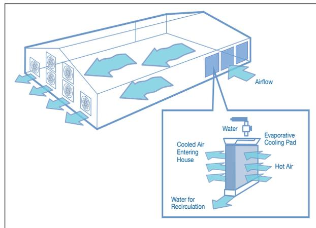
Figure 14: Pad cooling with tunnel ventilation
