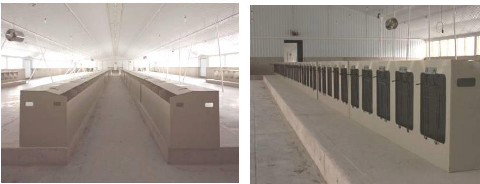
Figure 8: Plastic nest boxes placed on raised concrete platforms
